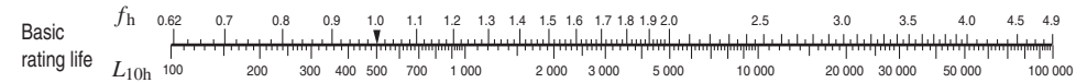
[Reference] Rotational speed ( n ) and its coefficients ( f n ), and service life coefficient ( f h ) and basic rating life ( L 10h )
